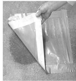
Fig. 3.1—When moisture is present after the plastic sheet test has been conducted, the surface feels cooler and is often a darker color (Kanare 2005).
