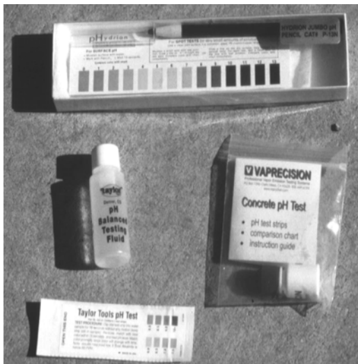
Fig. 4.2—pH indicators supplied with calcium chloride test kits. (Courtesy of Calvin McCall.)
