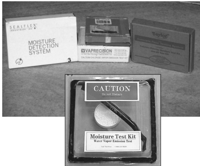
Fig. 3.5—Typical calcium chloride test kit for measuring moisture vapor emission rates. (Courtesy of Calvin McCall.)
