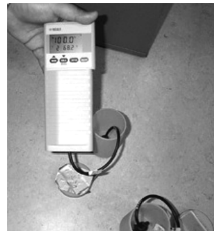
Fig. 3.8—Relative humidity measurement in a floor slab. (Courtesy of Peter Craig.)
