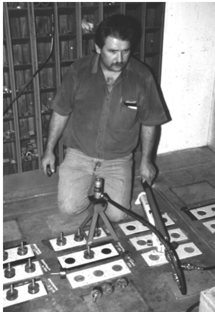
Fig. 8.2—Pulloff testing for vinyl composition tile placed on concrete slab with known moisture vapor emission rate (Suprenant 2003c).
