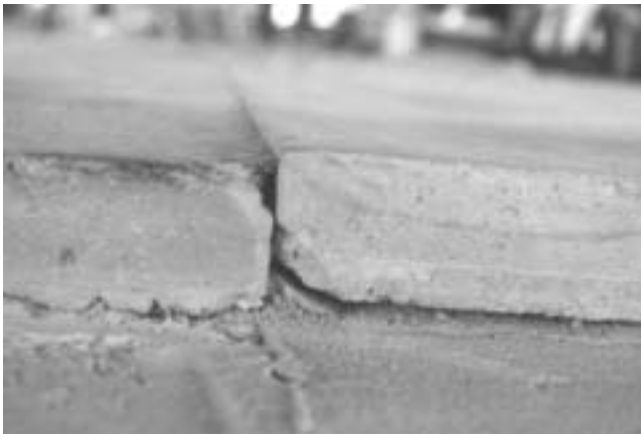
Fig. 11.12—Curling at joint in a 2 in. (50 mm) unbonded topping (courtesy of Eldon Tipping).
