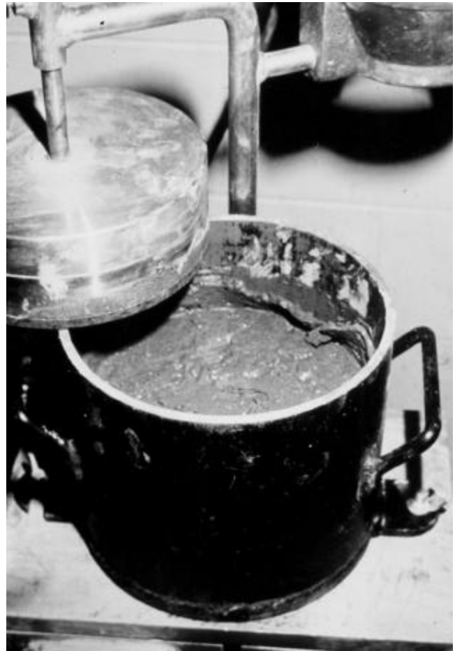
Fig. 6.3—Vebe consistency test time with ring of mortar on consolidated sample.
