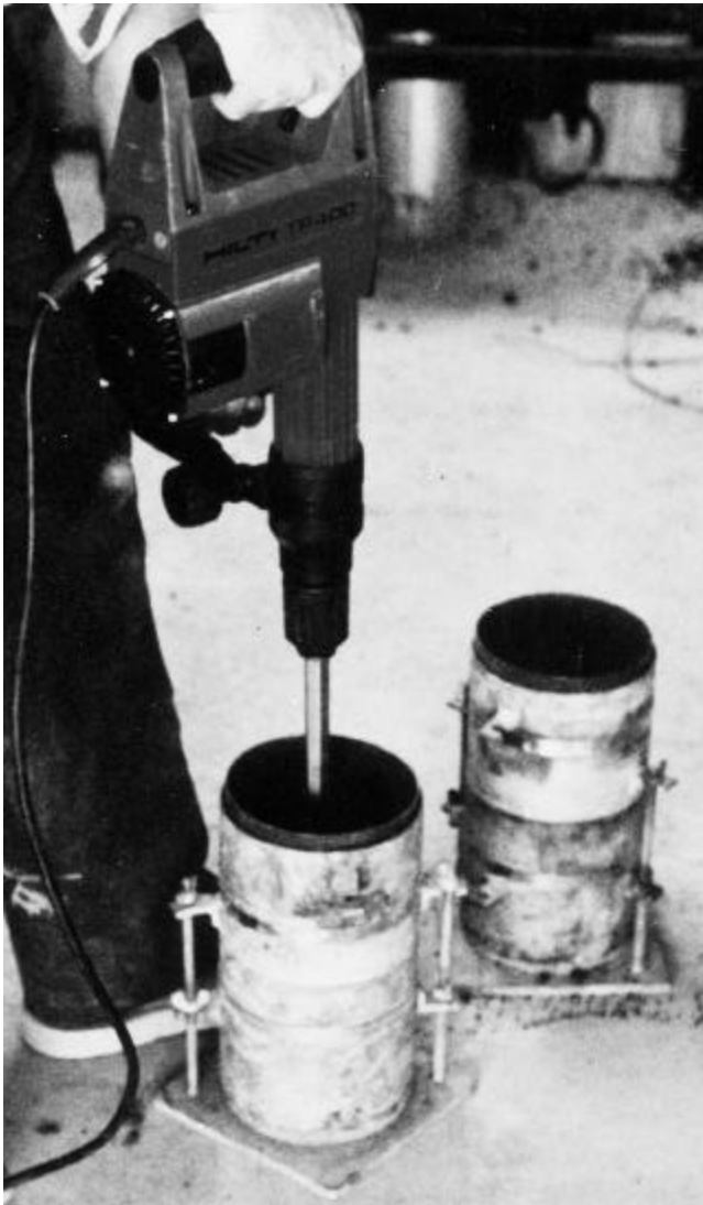
Fig. 6.7—Making RCC test cylinders with vibrating hammer.
