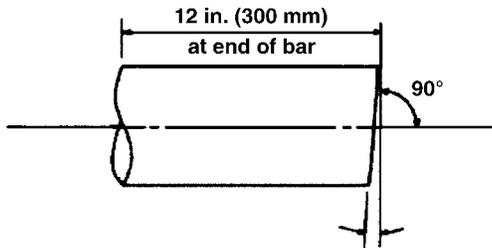
Maximum deviation from "square" to the end 12 in. [300 mm] of the bar (bar sizes #8 through #18 [#25 through #57]) should be 1-1/2° for compression connections.
